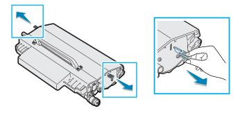
**9** Locate the transfer belt slots inside the printer, one on each side.
